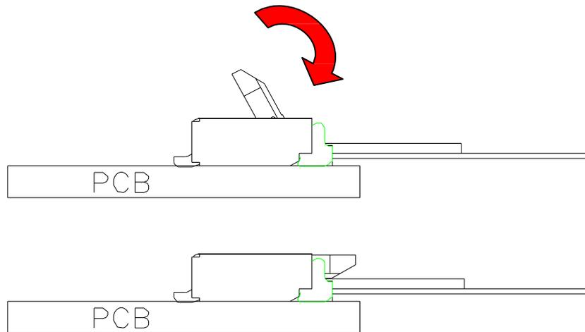
12.1.4 Lift up the actuator and pull out the FFC/FPC after the lock is released.
